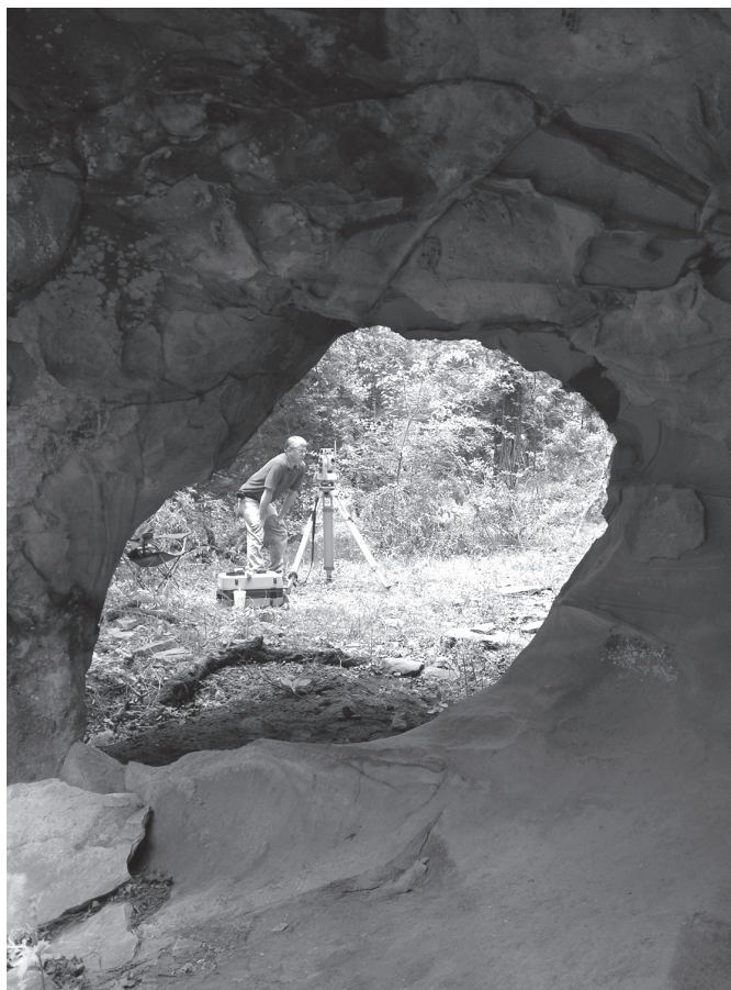
Tim Mulvihill using the Topcon Imaging Station to scan a rock art site.
