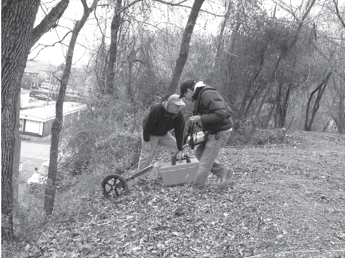
Tim Mulvihill and Dr. Jami Lockhart using ground penetrating radar at the Cavanaugh Mound in Fort Smith.
