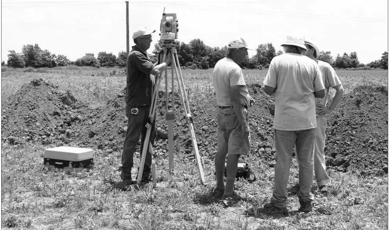
Tim Mulvihill setting up a robotic Total Station to map backhoe trench wall stratification at the Richard's Bridge site. Others in the photo: Marion Haynes, Larry Porter, Jami Lockhart.
