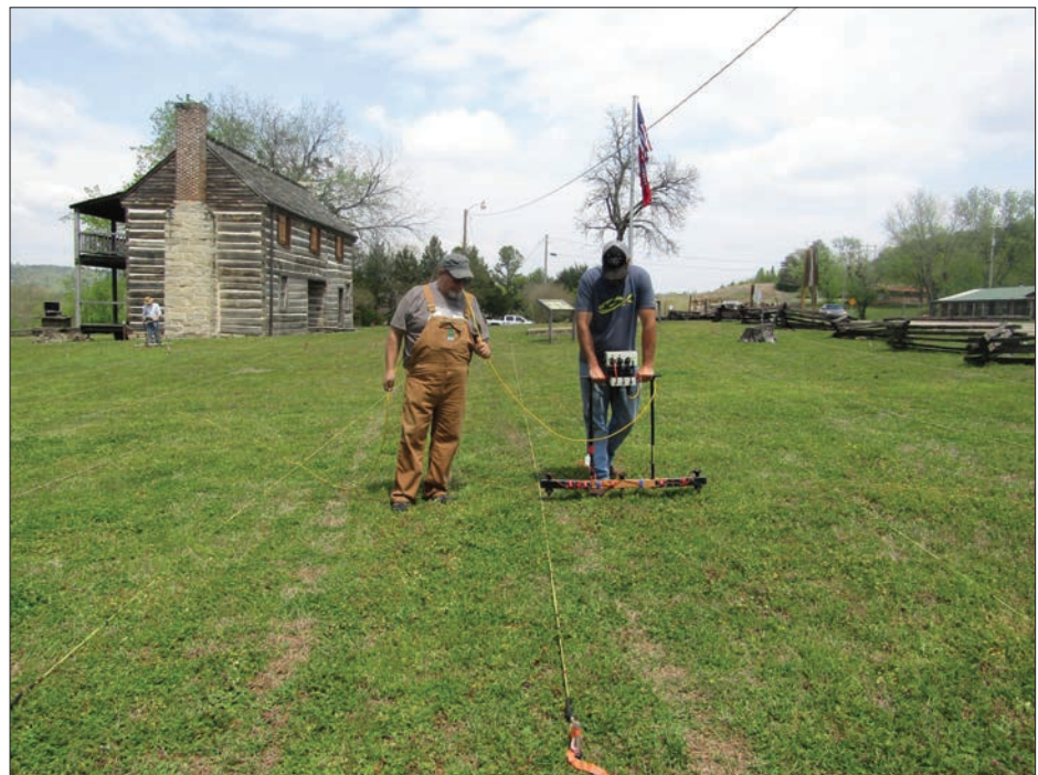
Jared Pebworth (left) and Michael Evans (right), with Dr. Jami Lockhart in the background near the house, collecting resistivity data at the Jacob Wolf House in Baxter County.
