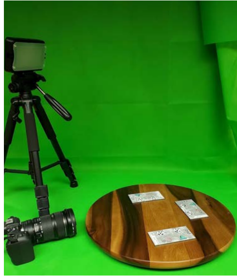
Set up at ARAS-WRI for creating 3D models of artifacts using photogrammetry.
