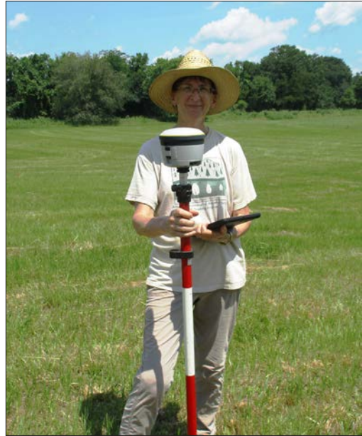
Mary Beth Trubitt using the station's new Trimble R2 and iPad to record locational data during a revisit to site 3HS22 in June 2021.
