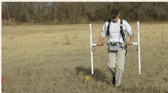
Gradiometer survey at a NW Arkansas site
